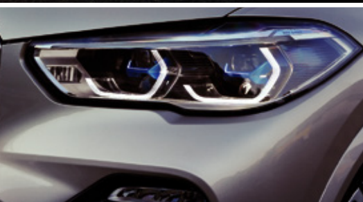
Adaptive LED headlights with BMW Laserlight incl. BMW Selective Beam
