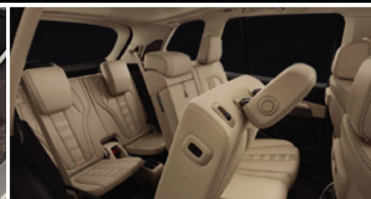
3 rd row seats with 2 nd row of seats incl. comfort entry and infinitely variable electric seat backrest tilt adjustment and fore-and aft adjustment incl. Comfort cushions.
